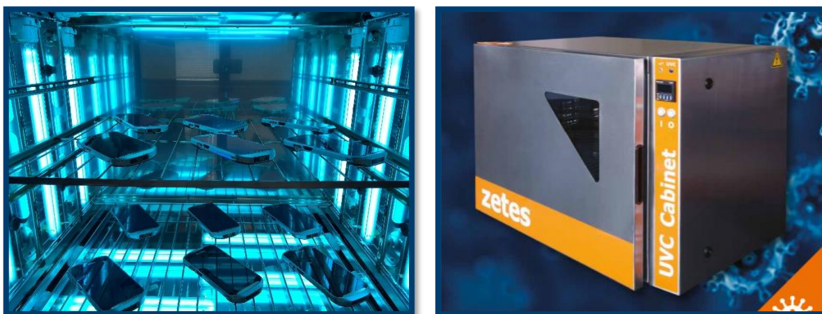
Figure 25: ZETES' UVC cabinet. Left: inside view with devices during a disinfection cycle. Right: outside view.
