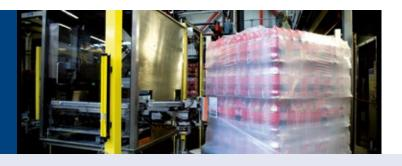
The MD-6000 is Zetes' high performance pallet labelling machine. It labels pallets on 1, 2, 3 or 4 sides and generates EDI-compliant messages to maximise customer satisfaction and optimise delivery times. The MD-6000 is steered by an industrial real-time controller capable of exchanging data between all the components of your packaging line.
