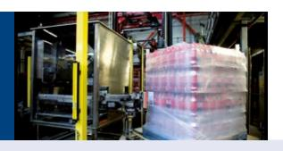
The MD-5000 is Zetes' high performance pallet labelling machine. It labels pallets on 1, 2 or 3 sides and generates EDI-compliant messages to maximise customer satisfaction and optimise delivery times. The MD-5000 is steered by an industrial real-time controller capable of exchanging data between all the components of your packaging line.
